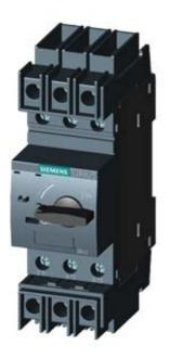
CIRCUIT-BREAKER SZ S00, FOR TRANSFORMER PROTECTION, WITH APPROBATION CIRCUIT-BREAKER UL 489. CSA C22.2 NO.5-02. A-RELEASE 2.5 A, N-RELEASE 52 A, SCREW CONNECTION, STANDARD SW. CAPACITY
