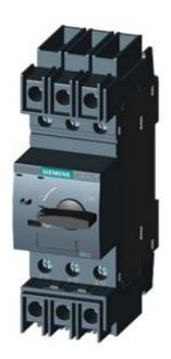
CIRCUIT-BREAKER SZ S00, FOR TRANSFORMER PROTECTION, WITH APPROBATION CIRCUIT-BREAKER UL 489. CSA C22.2 NO.5-02. A-RELEASE 1.25 A, N-RELEASE 26 A, SCREW CONNECTION, STANDARD SW. CAPACITY
