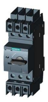
CIRCUIT-BREAKER SZ S00, FOR TRANSFORMER PROTECTION, WITH APPROBATION CIRCUIT-BREAKER UL 489. CSA C22.2 NO.5-02. A-RELEASE 0.5 A, N-RELEASE 10 A, SCREW CONNECTION, STANDARD SW. CAPACITY
