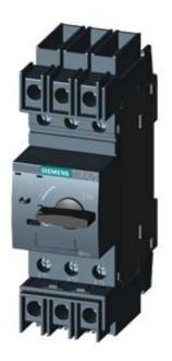
CIRCUIT-BREAKER SZ S00, FOR TRANSFORMER PROTECTION, WITH APPROBATION CIRCUIT-BREAKER UL 489. CSA C22.2 NO.5-02. A-RELEASE 1.6 A, N-RELEASE 33 A, SCREW CONNECTION, STANDARD SW. CAPACITY
