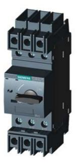
CIRCUIT-BREAKER SZ S00, FOR TRANSFORMER PROTECTION, WITH APPROBATION CIRCUIT-BREAKER UL 489. CSA C22.2 NO.5-02. A-RELEASE 0.4 A, N-RELEASE 8.2 A, SCREW CONNECTION, STANDARD SW. CAPACITY
