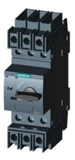
CIRCUIT-BREAKER SZ S00, FOR TRANSFORMER PROTECTION, WITH APPROBATION CIRCUIT-BREAKER UL 489. CSA C22.2 NO.5-02. A-RELEASE 0.25 A, N-RELEASE 5.2 A, SCREW CONNECTION, STANDARD SW. CAPACITY
