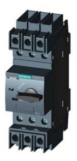
CIRCUIT-BREAKER SZ S00, FOR PLANT PROTECTION, WITH APPROBATION CIRCUIT-BREAKER UL 489. CSA C22.2 NO.5-02. A-RELEASE 6.3 A, N-RELEASE 82 A, SCREW CONNECTION, STANDARD SW. CAPACITY
