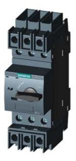
CIRCUIT-BREAKER SZ S00, FOR PLANT PROTECTION, WITH APPROBATION CIRCUIT-BREAKER UL 489. CSA C22.2 NO.5-02. A-RELEASE 5 A, N-RELEASE 65 A, SCREW CONNECTION, STANDARD SW. CAPACITY
