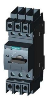
CIRCUIT-BREAKER SZ S00, FOR PLANT PROTECTION, WITH APPROBATION CIRCUIT-BREAKER UL 489. CSA C22.2 NO.5-02. A-RELEASE 0.8 A, N-RELEASE 10 A, SCREW CONNECTION, STANDARD SW. CAPACITY
