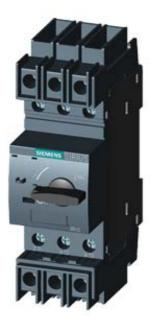
CIRCUIT-BREAKER SZ S00, FOR PLANT PROTECTION, WITH APPROBATION CIRCUIT-BREAKER UL 489. CSA C22.2 NO.5-02. A-RELEASE 0.25 A, N-RELEASE 3.3 A, SCREW CONNECTION, STANDARD SW. CAPACITY
