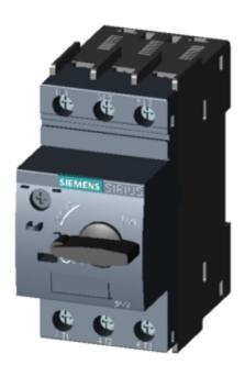
CIRCUIT-BREAKER SZ S00, FOR TRANSFORMER PROT. A-RELEASE 11...16A, N-RELEASE 286A, SCREW CONNECTION, STANDARD SW. CAPACITY
