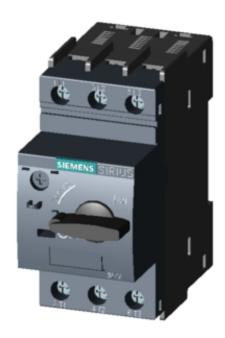
CIRCUIT-BREAKER SZ S00, FOR TRANSFORMER PROT. A-RELEASE 1.8...2.5A, N-RELEASE 52A SCREW CONNECTION, STANDARD SW. CAPACITY
