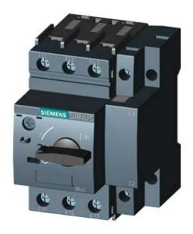
CIRCUIT-BREAKER SZ S00, FOR MOTOR PROTECTION, CLASS 10, W. OVERLOAD RELAY FUNCTION A-RELEASE4.5A...6.3A, N-RELEASE82A, SCREW CONNECTION, STANDARD SW. CAPACITY
