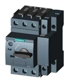
CIRCUIT-BREAKER SZ S00, FOR MOTOR PROTECTION, CLASS 10, W. OVERLOAD RELAY FUNCTION A-RELEASE 2.8A...4A, N-RELEASE 52A, SCREW CONNECTION, STANDARD SW. CAPACITY
