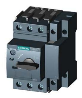
CIRCUIT-BREAKER SZ S00, FOR MOTOR PROTECTION, CLASS 10, W. OVERLOAD RELAY FUNCTION A-RELEASE1.8...2.5A, N-RELEASE33A, SCREW CONNECTION, STANDARD SW. CAPACITY
