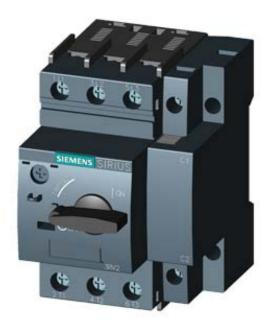
CIRCUIT-BREAKER SZ S00, FOR MOTOR PROTECTION, CLASS 10, W. OVERLOAD RELAY FUNCTION A-RELEASE 0.28...0.4A,N-RELEASE 5.2A SCREW CONNECTION, STANDARD SW. CAPACITY
