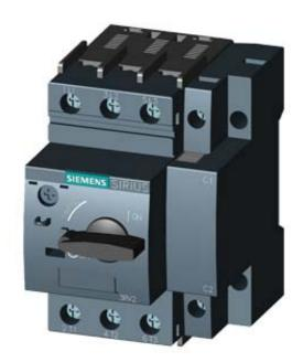
CIRCUIT-BREAKER SZ S00, FOR MOTOR PROTECTION, CLASS 10, W. OVERLOAD RELAY FUNCTION A-RELEASE0.35...0.5A, N-RELEASE6.5A SCREW CONNECTION, STANDARD SW. CAPACITY
