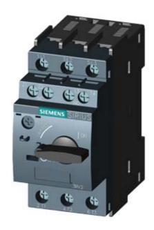
CIRCUIT-BREAKER SZ S00, FOR MOTOR PROTECTION, CLASS 10, A-RELEASE 5.5...8A, N-RELEASE 104A, SCREW CONNECTION, STANDARD SW. CAPACITY W. TRANSVERSE AUX. SWITCH 1NO+1NC
