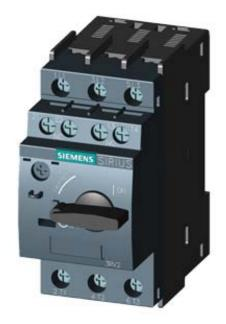
CIRCUIT-BREAKER SZ S00, FOR MOTOR PROTECTION, CLASS 10, A-RELEASE 2.8...4A, N-RELEASE 52A, SCREW CONNECTION, STANDARD SW. CAPACITY, W. TRANSVERSE AUX. SWITCH 1NO+1NC
