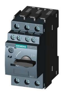
CIRCUIT-BREAKER SZ S00, FOR MOTOR PROTECTION, CLASS 10, A-REL. 0.18...0.25A, N-RELEASE3.3A SCREW CONNECTION, STANDARD SW. CAPACITY, W. TRANSVERSE AUX. SWITCH 1NO+1NC
