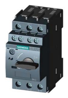
CIRCUIT-BREAKER SZ S00, FOR MOTOR PROTECTION, CLASS 10, A-REL. 0.55...0.8A, N-RELEASE10A, SCREW CONNECTION, STANDARD SW. CAPACITY, W. TRANSVERSE AUX. SWITCH 1NO+1NC
