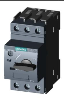
CIRCUIT-BREAKER SZ S00, FOR MOTOR PROTECTION, CLASS 10, A-REL. 0.55...0.8A, N-RELEASE10 A SCREW CONNECTION, STANDARD SW. CAPACITY
