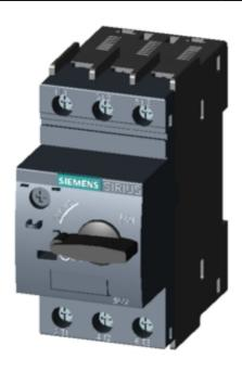
CIRCUIT-BREAKER SZ S00, FOR MOTOR PROTECTION, CLASS 10, A-RELEASE 0.11...0.16A, N-RELEASE2.1A SCREW CONNECTION, STANDARD SW. CAPACITY
