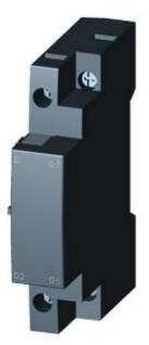
UNDERVOLTAGE RELEASE, AC 230V/50HZ, AC 240V/60HZ, WITH LEADING AUX. CONTACTS 2NO, W. SCREW CONNECTION, FOR CIRCUIT-BREAKERS, SZ S00/S0
