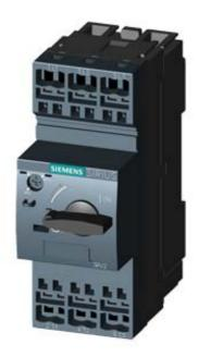
CIRCUIT-BREAKER SZ S0, FOR TRANSFORMER PROT. A-RELEASE 20...25A, N-RELEASE 400A, SPRING-L. CONNECTION, STANDARD SW. CAPACITY
