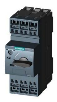
CIRCUIT-BREAKER SZ S0, FOR TRANSFORMER PROT. A-RELEASE 17...22A, N-RELEASE 364A, SPRING-L. CONNECTION, STANDARD SW. CAPACITY
