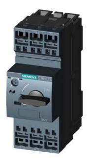
CIRCUIT-BREAKER SZ S0, FOR TRANSFORMER PROT. A-RELEASE 14...20A, N-RELEASE 325A, SPRING-L. CONNECTION, STANDARD SW. CAPACITY
