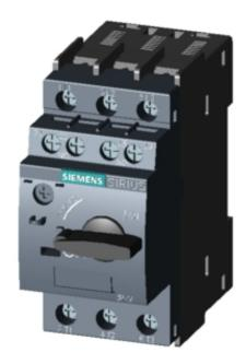
CIRCUIT-BREAKER SZ S0, FOR MOTOR PROTECTION, CLASS 10, A-RELEASE 34...40A, N-RELEASE 480A, SCREW TERMINAL, STANDARD SWITCHING CAPACITY, W. TRANSVERSE AUX. SWITCH 1NO+1NC
