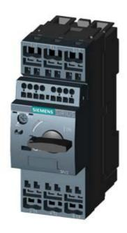
CIRCUIT-BREAKER SZ S0, FOR MOTOR PROTECTION, CLASS 10, A-RELEASE 11...16A, N-RELEASE 208A, SPRING-L. CONNECTION, STANDARD SW. CAPACITY, W. TRANSVERSE AUX. SWITCH 1NO+1NC
