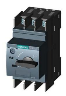
CIRCUIT-BREAKER SZ S00, FOR MOTOR PROTECTION, CLASS 10, A-RELEASE 9..12.5A, N-RELEASE 156A, RING CABLE LUG CONNECTION, STANDARD SW. CAPACITY
