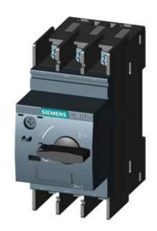
CIRCUIT-BREAKER SZ S00, FOR MOTOR PROTECTION, CLASS 10, A-RELEASE 7...10A, N-RELEASE 130A, RING CABLE LUG CONNECTION, STANDARD SW. CAPACITY
