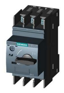
CIRCUIT-BREAKER SZ S00, FOR MOTOR PROTECTION, CLASS 10, A-RELEASE 4.5...6.3A, N-RELEASE 82A RING CABLE LUG CONNECTION, STANDARD SW. CAPACITY
