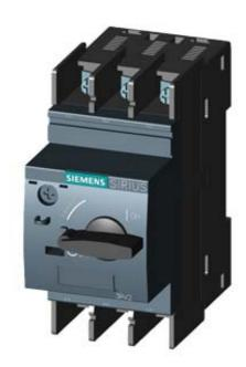
CIRCUIT-BREAKER SZ S00, FOR MOTOR PROTECTION, CLASS 10, A-RELEASE2.2...3.2A, N-RELEASE 42A, RING CABLE LUG CONNECTION, STANDARD SW. CAPACITY
