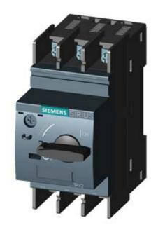
CIRCUIT-BREAKER SZ S00, FOR MOTOR PROTECTION, CLASS 10, A-REL.1.8...2.5A, N-RELEASE 33A, RING CABLE LUG CONNECTION, STANDARD SW. CAPACITY
