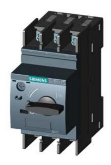
CIRCUIT-BREAKER SZ S00, FOR MOTOR PROTECTION, CLASS 10, A-REL. 0.9...1.25A, N-RELEASE16A, RING CABLE LUG CONNECTION STANDARD SW. CAPACITY
