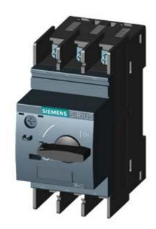
CIRCUIT-BREAKER SZ S00, FOR MOTOR PROTECTION, CLASS 10, A-REL. 0.18...0.25A, N-RELEASE3.3A RING CABLE LUG CONNECTION STANDARD SW. CAPACITY
