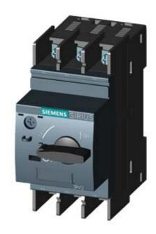
CIRCUIT-BREAKER SZ S00, FOR MOTOR PROTECTION, CLASS 10, A-REL. 0.14...0.2A, N-RELEASE2.6A, RING CABLE LUG CONNECTION STANDARD SW. CAPACITY
