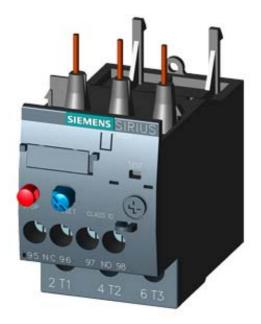
OVERLOAD RELAY 3.5...5.0 A FOR MOTOR PROTECTION SZ S0, CLASS 10, F. MOUNTING ONTO CONTACTOR MAIN CIRCUIT: SCREW TERMINAL AUX. CIRCUIT: SCREW TERMINAL MANUAL-AUTOMATIC-RESET
