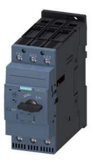
CIRCUIT BREAKER, SIZE S2, FOR MOTOR PROTECTION, CLASS 10, A-RELEASE 20...25A, N-RELEASE 325A, SCREW TERMINAL, INCREASED SWITCHING CAPACITY
