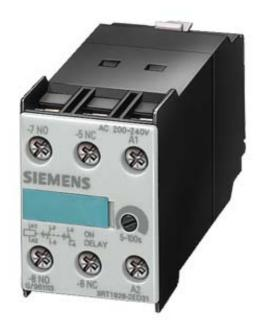
SOLID-STATE, TIME-DELAYED AUXILIARY SWITCH BLOCK SETTING RANGE 0.05 S...1 NO, AC 100...127 V, 1NO + 1NC, ON-DELAY, FOR MOUNTING ONTO CONTACTORS SIZE S0...S12
