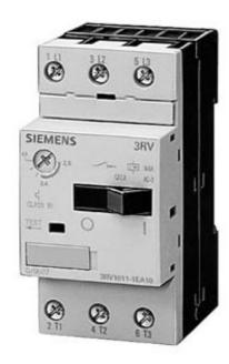
CIRCUIT-BREAKER SIZE S00, FOR MOTOR PROTECTION, CLASS 10, A-REL.1.1...1.6A, N-REL. 21A, SCREW TERMINAL, STANDARD SWITCHING CAPACITY
