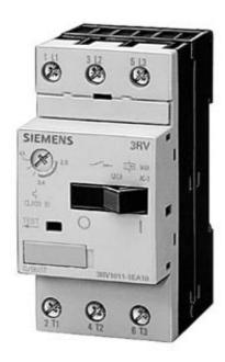
CIRCUIT-BREAKER SIZE S00, FOR MOTOR PROTECTION, CLASS 10, A-REL. 9...12A, N-REL. 156A, SCREW TERMINAL, STANDARD SWITCHING CAPACITY
