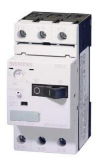
CIRCUIT-BREAKER SIZE S00, FOR MOTOR PROTECTION, CLASS 10, A-REL.0.35...0.5A, N-REL.6.5A SCREW TERMINAL, STANDARD SWITCHING CAPACITY
