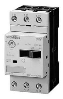
CIRCUIT-BREAKER SIZE S00, FOR MOTOR PROTECTION, CLASS 10, A-REL. 5.5...8A, N-REL. 104A, SCREW TERMINAL, STANDARD SWITCHING CAPACITY
