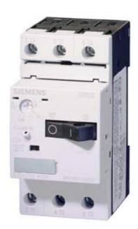
CIRCUIT-BREAKER SIZE S00, FOR MOTOR PROTECTION, CLASS 10, A-REL.0.45...0.63A,N-REL.8.2A SCREW TERMINAL, STANDARD SWITCHING CAPACITY
