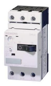
CIRCUIT-BREAKER SIZE S00, FOR MOTOR PROTECTION, CLASS 10, A-REL.0.28...0.4A,N-REL.5.2A, SCREW TERMINAL, STANDARD SWITCHING CAPACITY
