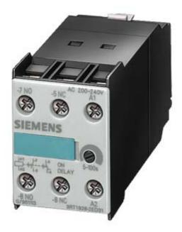
SOLID-STATE, TIME-DELAYED AUXILIARY SWITCH BLOCK SETTING RANGE 0.5 S...10 S, AC/DC 100...127 V, 1NO + 1NC, OFF-DELAY, FOR MOUNTING ONTO CONTACTORS SIZE S0...S12
