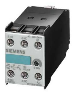
SOLID-STATE, TIME-DELAYED AUXILIARY SWITCH BLOCK SETTING RANGE 0.05 S...1 NO, AC/DC 100...127 V, 1NO + 1NC, OFF-DELAY, FOR MOUNTING ONTO CONTACTORS SIZE S0...S12
