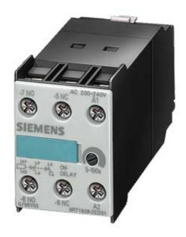
SOLID-STATE, TIME-DELAYED AUXILIARY SWITCH BLOCK SETTING RANGE 0.5 S...10 S, AC/DC 24 V, 1NO + 1NC, OFF-DELAY, FOR MOUNTING ONTO CONTACTORS SIZE S0...S12
