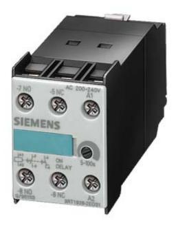
SOLID-STATE, TIME-DELAYED AUXILIARY SWITCH BLOCK SETTING RANGE 5 S...100 S, AC 200...240 V, 1NO + 1NC, ON-DELAY, FOR MOUNTING ONTO CONTACTORS SIZE S0...S12
